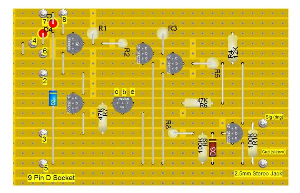
The layout was compressed to fit into an aluminium "u" box measuring 75x50x25mm.
